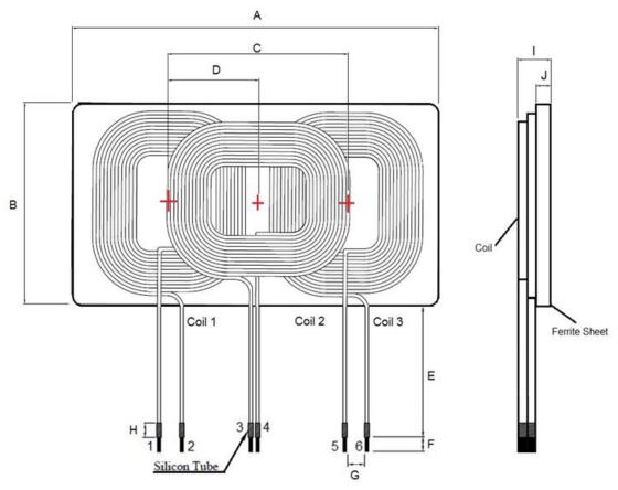
Note: Pin 1,4,5-Red Silicon Tube, Pin 2,3,6-Black Silicon Tube
